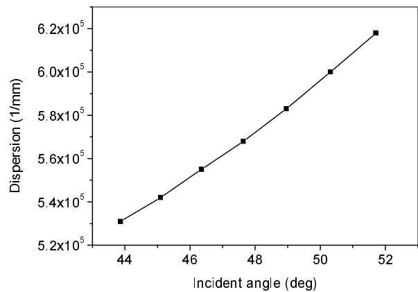
Figure 2 Angular dispersion efficiency as a function of incident angle for RAP crystal.
