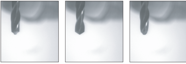
Fig. 2 Sample images of a sharp drilling tool
